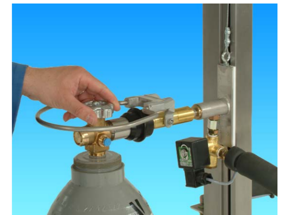
Slowly open CO2 valve. The CO2 cylinder is now ready to be filled. 6
