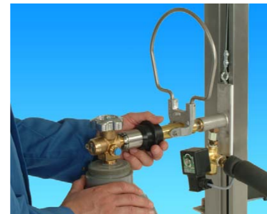
Slide rubber ring towards valve. 2
